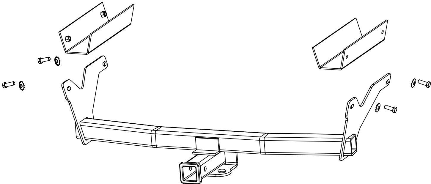
1. Locate and remove the two plastic weld nut plugs in the outside vertical surface of frame rail on both the passenger and driver's side using a small flat screwdriver. Return the four plugs to the vehicle owner.
