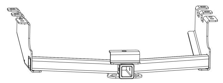
Note: Factory installed steel step bumper and brackets must be used in conjunction with hitch.
