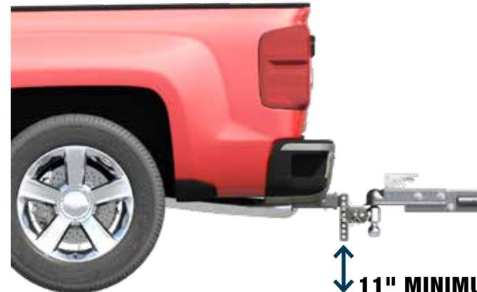
Ensure that you have chosen a hitch that provides enough vertical adjustment to allow your trailers to tow as level as possible while providing enough ground clearance.
