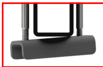
FIGURE D7: View showing an incorrectly tightened frame clamp.
