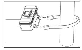
Freespool the hook and winch rope out to the load and secure using the second supplied strap. ALWAYS be sure that the hook latch closes around the loop straps. Latch closed with strap loops inserted in the hook. See **Figure 7.**
