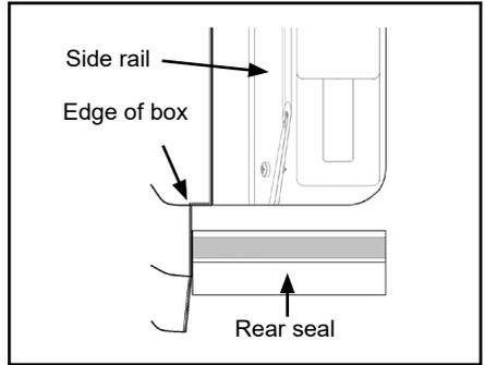
B. Mark seal leg and then cut notch in seal.
