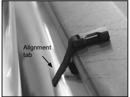
C. Slide left tension adjuster until it engages under side rail (see Step 5F). Push bar back and forth to line up holes. Do not turn adjustment wheel. Insert bolt from top and nut from bottom.
