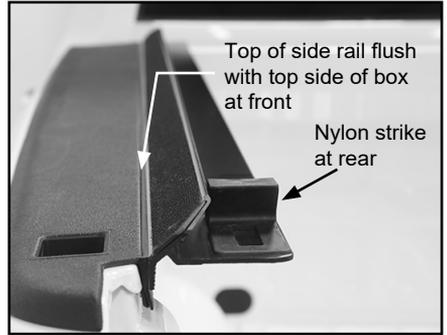
B. At front, adjust top of side rail until flush with top of box and hold with assistance of another person or a spring clamp.
